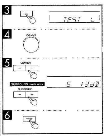
Press TEST to output a test signal
